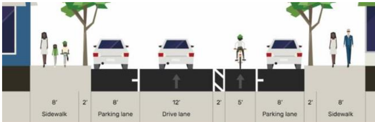
FIGURE 8A: MAIN STREET TYPICAL SECTION (ALT 1A)
