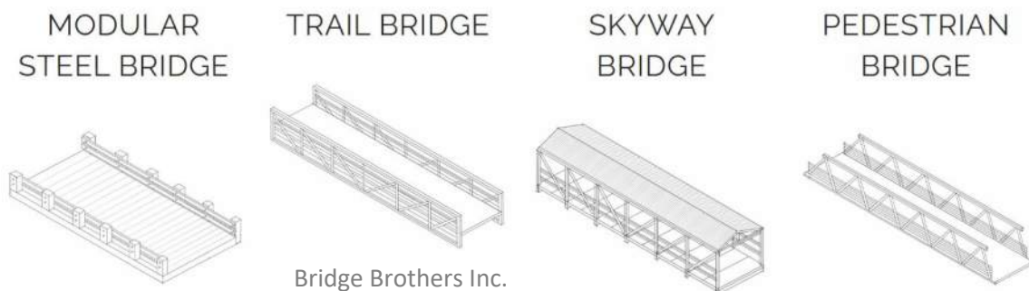
FIGURE 4: ALTERNATE PED BRIDGE CONFIGURATIONS
